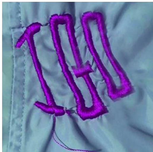
Fig. 2.19 – Puckering of Embroidery due to improper or no framing
