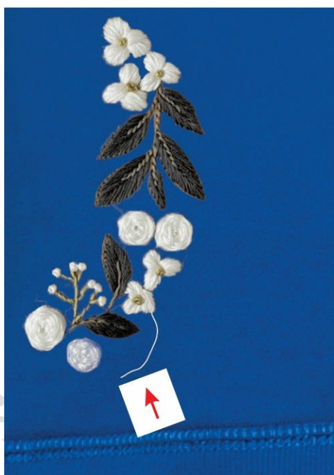
Fig. 3.13 – Identification and marking of embroidery defects
