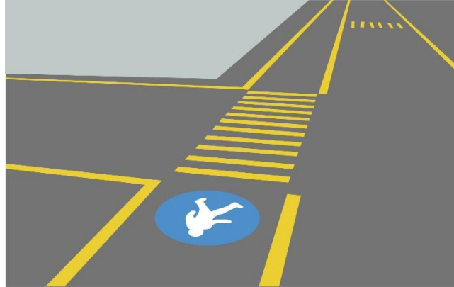
Fig. 5.3 – Yellow Demarcation for Pedestrian Pathway
