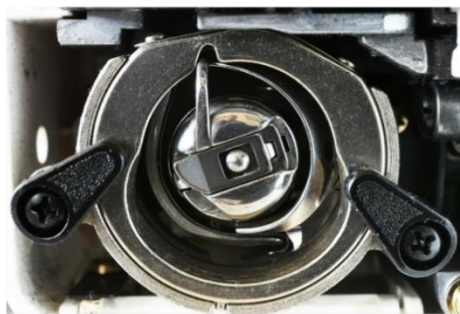
Fig. 3.1 – Bobbin related problems: Bobbin should be placed properly in the winder
